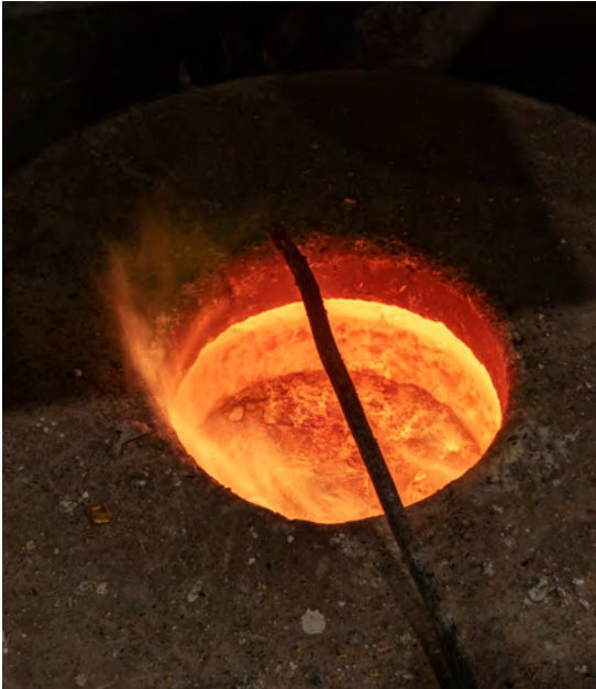
Bronze, an alloy typically composed of copper and tin, is melted in a furnace until it becomes a liquid at around 950°C (1742°F)
