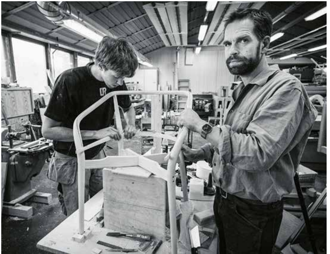
Thomas E. Alken in the workshop with a prototype for a chair with front legs, armrests and back all made from one piece of pre-compressed bent wood.
