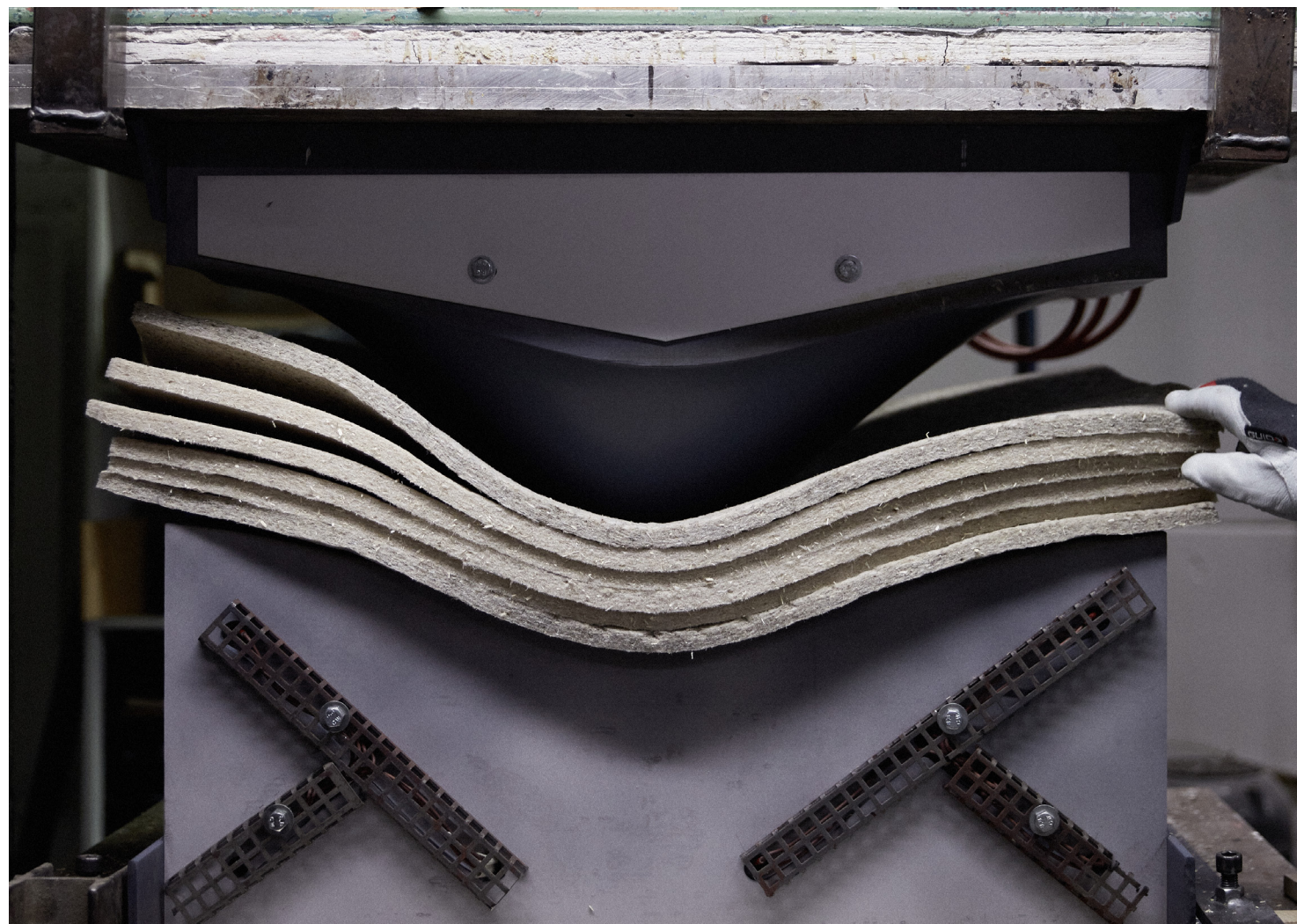
Mat Chair shell in the compression process
